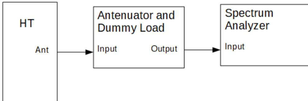
**Note :** Requires an sma (male or female) to SO-239 adapter at HT antenna port. Patch cables may require type N or BNC connectors.
