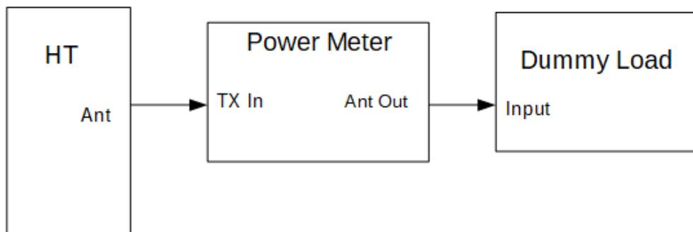
**Note: Requires an sma (male or female) to SO-239 adapter at HT antenna port**
